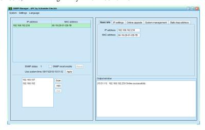
You can modify IP setting, online upgrade, password management, and static trap address setting in SNMP Manager interface. It is necessary to enter password for any modification. The default password is 12345678.
