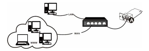
When the network interface cable is connected, the SNMP Card will attempt to obtain an IP address via DHCP. See "Configuration methods" on page 6.
