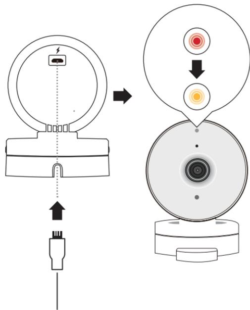
Plug the included USB Power Adapter into the back of the camera. Wait until the LED at the front changes from red to blinking orange.
