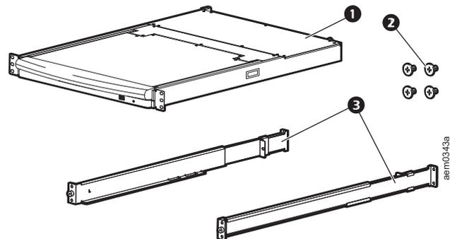
4. Slide the rear attachment sliding brackets along the slide bars until they contact the rear of the KVM Rack LCD. Use the supplied screws to attach the bars to the rear of the KVM Rack LCD switch. Fully tighten these screws.
