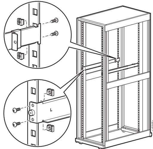
3. Slide the KVM Rack LCD (1) onto the support flanges (3). Use the screws (2) supplied to loosely attach the front of the KVM Rack LCD to the front of the rack.
