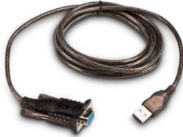
USB to Serial Adapter          | 203-182-100                                          | <p>The USB to RS-232 adapter connects to the printer USB host (type A) port and provides serial RS-232 (female DB9) connectivity. Cable length is 1.8m. Serial flow control: XON/XOFF, RTS/CTS. (All models, RoHS)</p>                                                                                                                                                                        |
