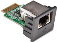
Ethernet (IEEE 802.3) Module | 203-183-210 (PC23d)<br>203-183-410 (PC43d,<br>PC43t) | <p>The user installable IEEE 802.3 Ethernet module installs on the back of the printer (in place of the cover plate) and supports 10Base-T and 100Base-TX LAN communications. RJ45 CAT 5 cables up to 100m in length are supported. (PC23 Ethernet module has light case and PC43 Ethernet module has dark case, RoHS).</p> <p>Network Protocols Supported: TCP/IP, FTP, SNMP, LPR, HTTP.</p> |
