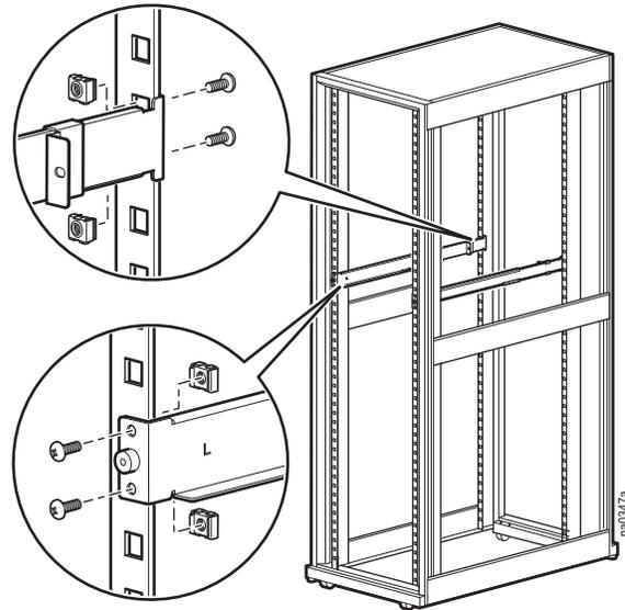
3. Slide the Rack LCD Console (1) onto the support flanges (3). Use the M4 x 6 screws (2) supplied to loosely attach the front of the Rack LCD Console to the front of the rack.
