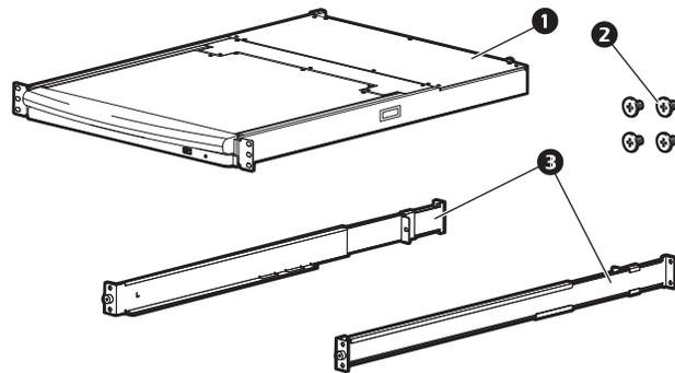
4. Slide the rear attachment sliding brackets along the slide bars until they contact the rear of the Rack LCD Console. Use the supplied M4 x 6 screws to attach the bars to the rear of the Rack LCD Console switch. Fully tighten these screws.
