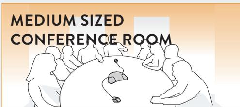
Place the expansion microphones on each side of the Konftel 300/300IP/300IPx. Expansion microphones effectively double the voice pickup range. Together, the microphones ensure optimal voice pickup in meeting rooms.
